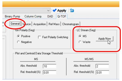
This will send the HPLC solvent flow into the mass spectrometer.
