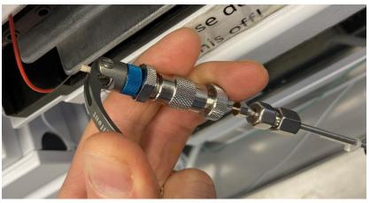
Then screw the plastic fitting into the exit end of the column (this fitting should be tight):
