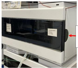
Push the button on the side of the autosampler to open the door.
