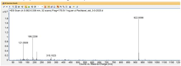
You should see the reference mass ions in the background spectrum, and they should be the correct exact mass. In positive ion mode, the exact m/z values are 121.0509 and 922.0098. In negative ion mode, the exact m/z values are 112.9856 and 1033.9881.
