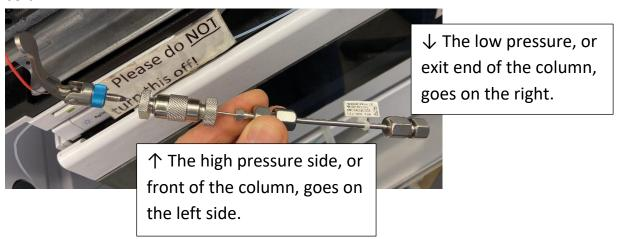
Screw the front of the column into the high-pressure fitting until you just feel the column bottom out. Do not over-tighten. Just light pressure. Then put the lever down.
