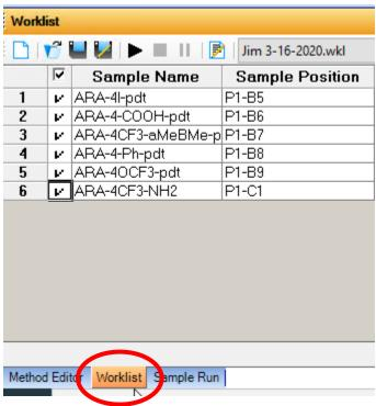
To set up the worklist, you will need to enter one row for each sample that you want to run. In each row, you need to specify the Sample Position, which is where you placed the sample in the autosampler.
