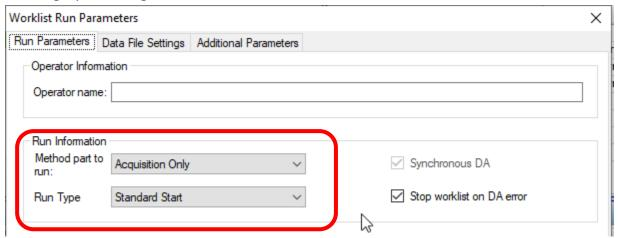
Make sure that "Method part to run:" is set to "Acquisition Only", and "Run Type" is set to "Standard Start".
