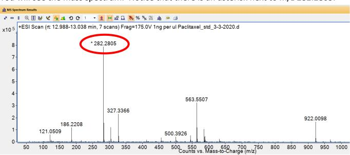
The asterisk means that this m/z peak is saturated. The signal was too large, because the sample was too concentrated. When this happens, the m/z value will not be as accurate as is could be.
