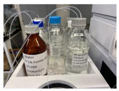
If the acetonitrile bottle is low on solvent, please replace the bottle with one of the spare full bottles of acetonitrile. Then update the solvent level in the software so that the data system will know how much solvent is available.
