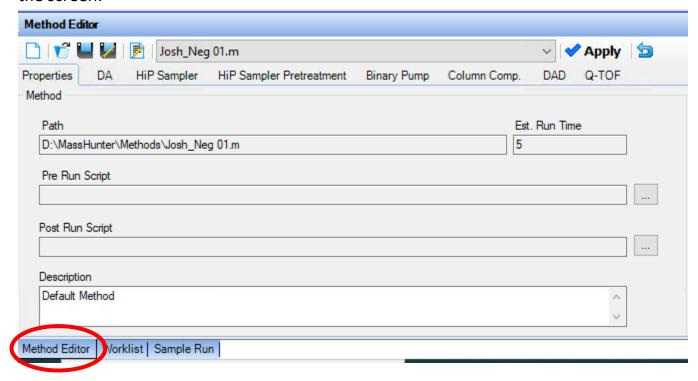
In the method editor, there are tabs for each piece of hardware in the system: The Autosampler, the Binary Pump, the Column Compartment, the UV-VIS Diode Array Dectector (DAD), and the Q-TOF.
