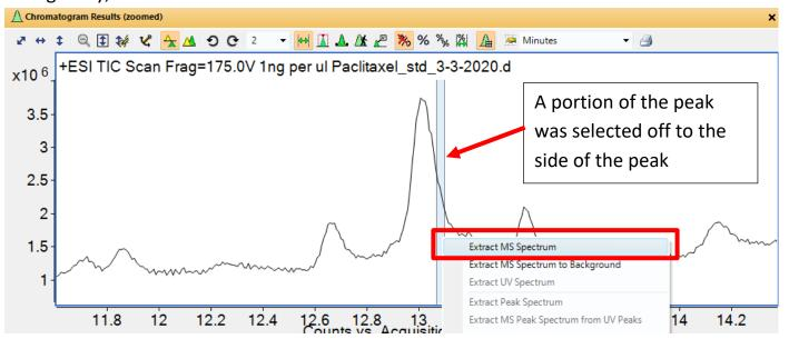
Right-click to get a menu, and click on "Extract MS Spectrum". The resulting spectrum in this case is not saturated (no asterisk next to any m/z values):
