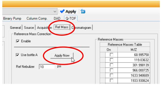
This will send the Bottle A reference mass solution into the mass spectrometer. You should then see the reference mass ions in the mass spectrum window. In positive ion mode, these reference ions will be m/z 121 and m/z 922. In negative ion mode, these reference ions will be m/z 112.9 and m/z 1034.
