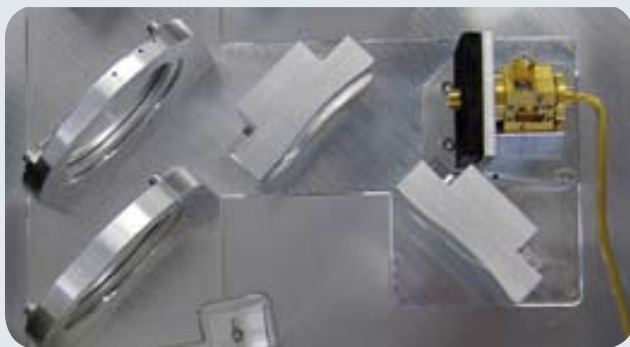
Quasi optical front-end of ELEXSYS-II E780
