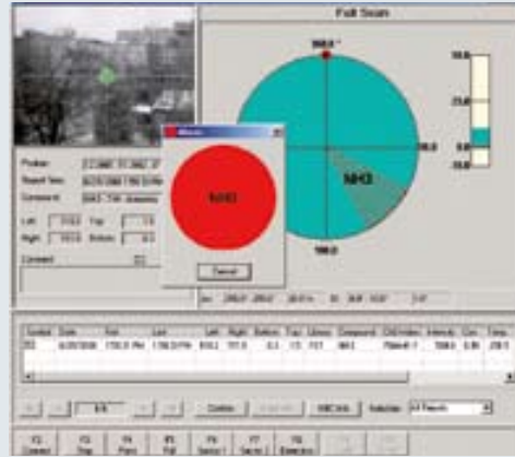
RAPID Control software with alarm window, on-line video picture and function keys for fast access to all system operation parameters.
