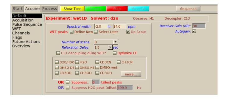
If Select Later was checked, the panel shown below opens up after the scout spectrum is measured. Expand the spectrum and select peaks in the same manner described for presat. Remember to click on [Acquire] (do not type go or ga) to start the acquisition.
