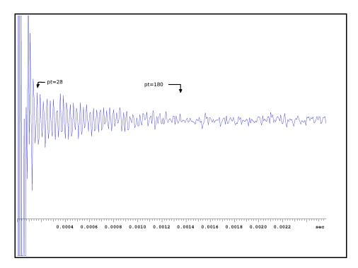
Backward linear prediction can be used to calculate and substitute the corrupted data points. First we need to know how many points are bad. Display the FID with df, expand the region at the beginning of the FID and position the cursor where you think the bad points end and type UMpoint. This macro displays, in the
