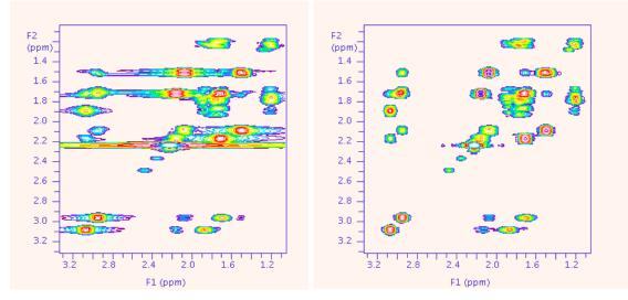
Vnmrj always tries to add appropriate forward linear prediction parameters during setup of a 2D experiment, so you should not worry about them. But if you need or want to modify them, they are found in the **Process**, **More 2D** parameter panel.
