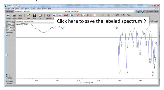
3) The labels on some of the tallest peaks may not appear on the screen. This can be rectified by clicking on the Full Screen button on the toolbar.
