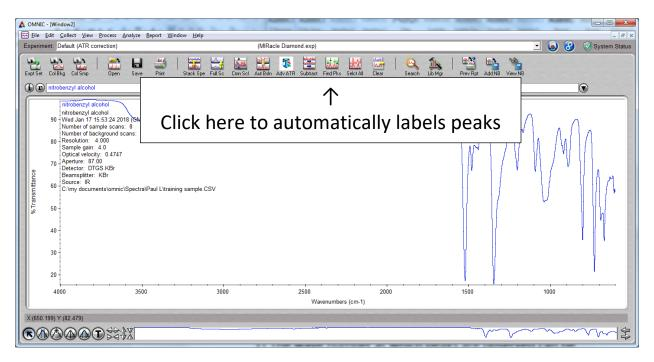
2) When the Find Peaks button is clicked, a horizontal line appears on the spectrum, indicating the threshold value for defining a peak. Click with the tip of the cursor to reposition this threshold line. When the desired position is determined, click on the Replace button in the upper right corner of the page to save the labeled spectrum.
