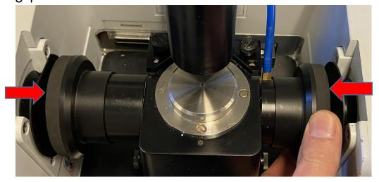
3) Then carefully lift up and out the ATR accessory:
