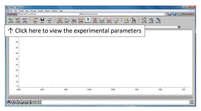
2) The default parameters for a standard characterization spectrum are 8 scans and a resolution of 4. The number of scans can be chosen by entering the desired value. Resolution values are chosen from the drop down menu.
