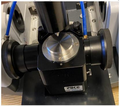
4) Insert the baseplate for Transmission IR. Note the alignment pins on the front and the back:
