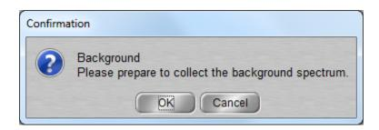
3. After confirmation, the instrument begins to collect data. The steps that the instrument takes can be viewed in the bottom left corner of the screen. First, a couple of setup processes are completed, then a countdown of the chosen number of scans begins (1 of 8, 2 of 8, etc.).
