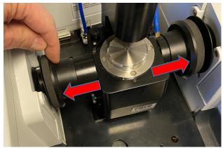
The cover remains open when the ATR accessory is installed. The carbon dioxide and water vapor are purged out of the inside of the accessory.
