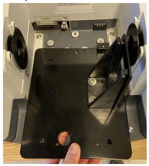
3) Insert the ATR accessory and base plate. Note the two alignment pins in the front and the back:
