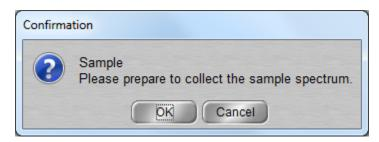
5. After confirmation, the instrument begins to collect data. The steps that the instrument takes can be viewed in the bottom left corner of the screen. First, a couple of setup processes are completed, then a countdown of the chosen number of scans begins (1 of 8, 2 of 8, etc.). When the collection is complete, the spectrum is displayed and you are prompted to save the data to the currently opened window. If the data are acceptable, click "Yes" to save the spectrum.
