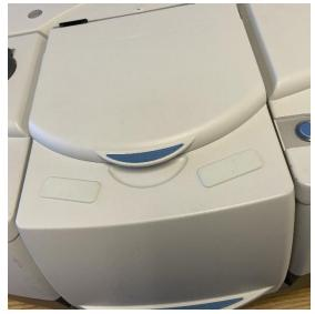
Please note: The sample compartment door must remain closed when doing transmission IR. It should be opened only briefly to insert a sample, and then closed again. After the cover has been open, you need to wait several minutes for the nitrogen gas to purge out traces of carbon dioxide and water vapor.
