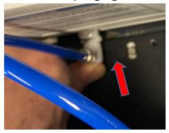
5) Push out both tube extensions so that there is no air gap:
