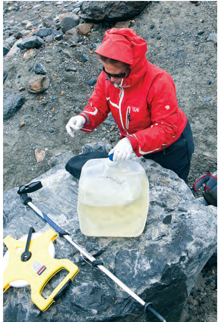
Sarah Aciego (Asst. Professor) setting up the chemistry in the carboy of filtered water for the iron co-precipitation of the uranium.
